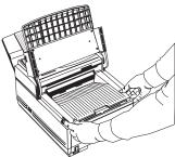
CAUTION: Never expose the image drum unit to light for more than 5 minutes. Never expose the image drum unit to direct sunlight. Always hold the image drum unit
